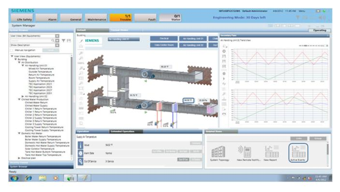
Desigo CC's User Interface provides effective system operation and control. It presents well arranged, relevant information to the user and is ready for interaction without any overlapping windows. The user views can be customized to allow for personal preferences with multiple sources of information streamed to one screen, increasing efficiency while saving time and money.
